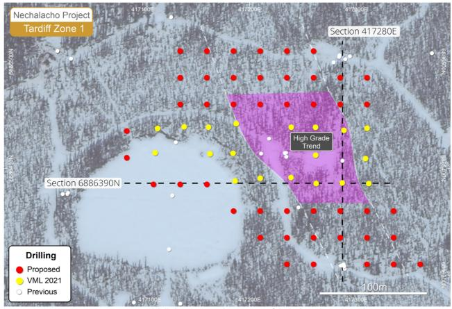
Figure 3 – 2022 proposed drill plan targeting the extension of the high grade north-south trend
